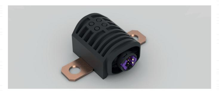
Pyrotechnical safety device, used for secure electrical separation of the conductor. Separation is done pyrotechnically. The CB 60 has to be triggered for activation in the event of an accident.
